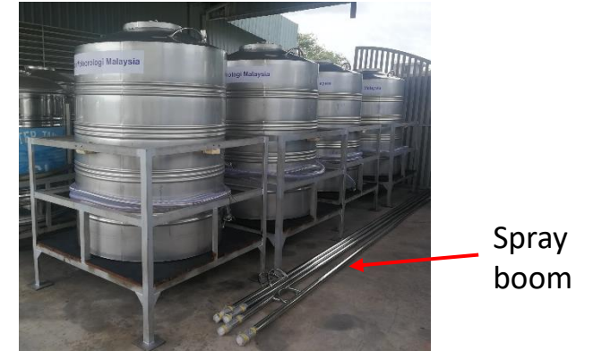
Fig. 3 Wet seeding equipment
